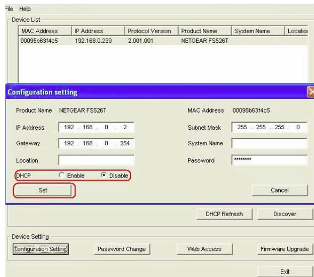
**Figure 3-4: Assigning the switch a static IP address**
